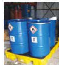
Barrels for used oils stored indoors. The used oils are sent for recycling to the respective Alternative Management System.
