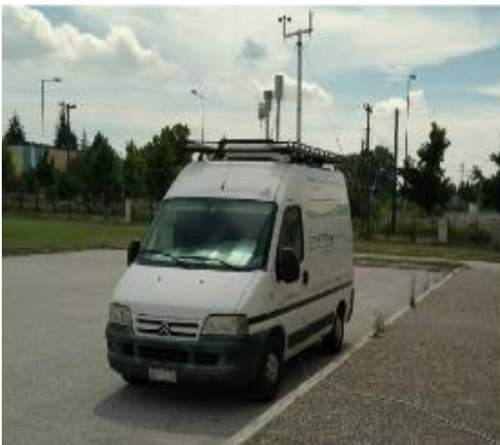
Figure 26: Mobile air quality monitoring station at Thessaloniki (SKG) airport
